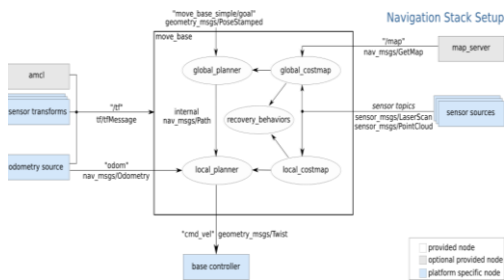
Fig. 97. ROS Navigation Grafiksel Model [16]
